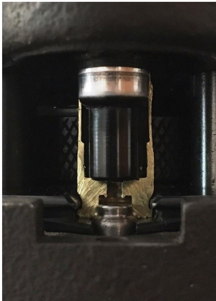
Figure 23: Cross-section of properly adjusted Swage Rod
