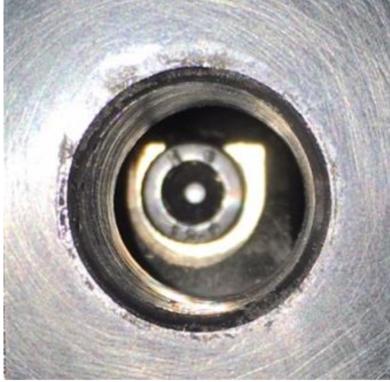
Figure 41: Socket head cap screw lined up with access hole.
