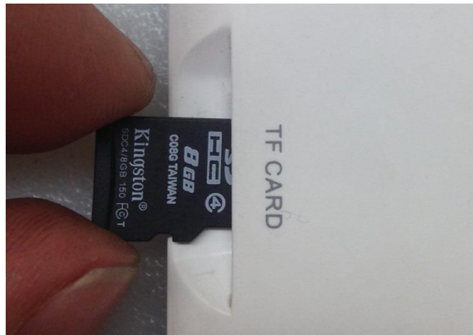
Figure 37: Orientation of Micro SD card
