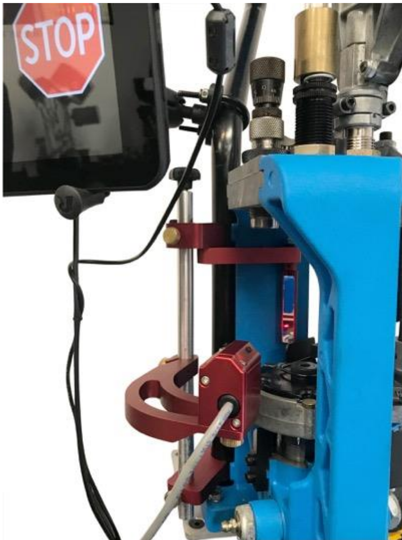
Figure 6: Lining Up Laser with Mirror (Crude Adjustment)
