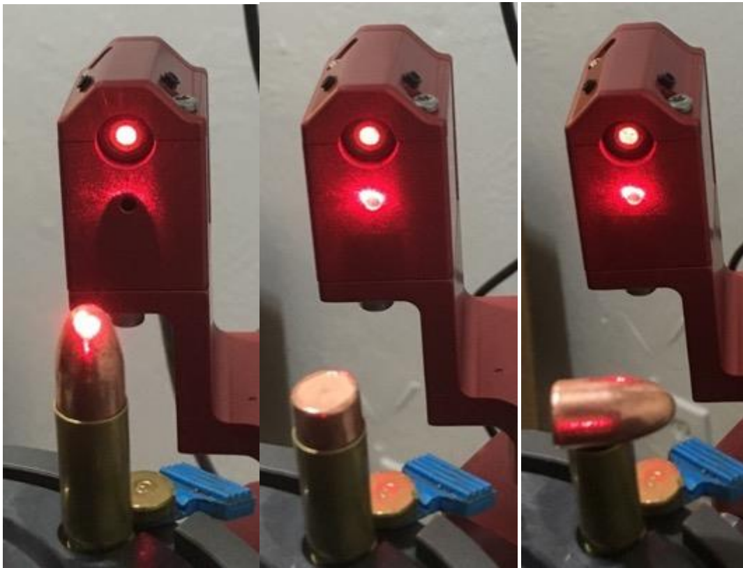
Figure 11: Bullet Properly Oriented - Beam Interrupted (Left) vs. Bullets Improperly Oriented – Beam not interrupted (Center and Right)
