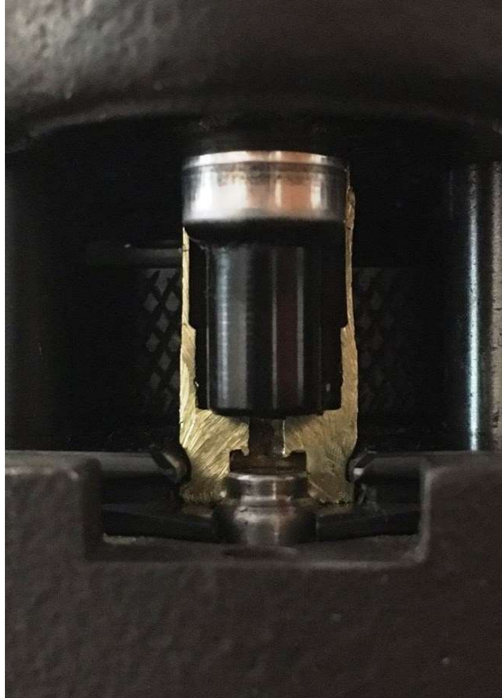
Figure 25: Cross-section of properly adjusted Swage Rod
